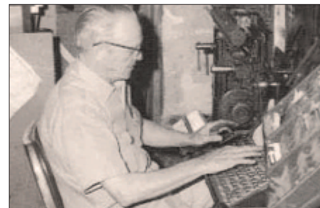
The newspaper's production changed with the times. An employee, above left, sets type, letter by letter, with the linotype machine. The 'set' page would then be put on the press. Years later, Regina
